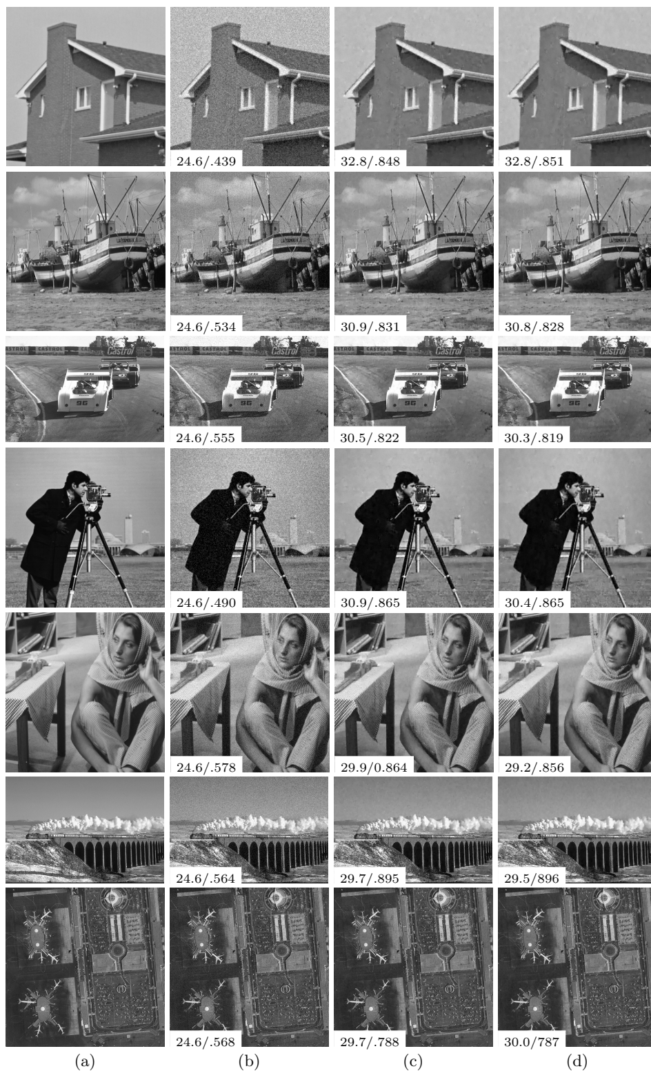
Fig. 2. Denoising results: (a) original, (b) noisy images with \sigma^2 = 15 , (c) results with truncated EM model, (d) results LR-COMP model with PSNR/SSIM. Similar denoising performances are obtained with LR-COMP with a compressed database 250 times smaller.
