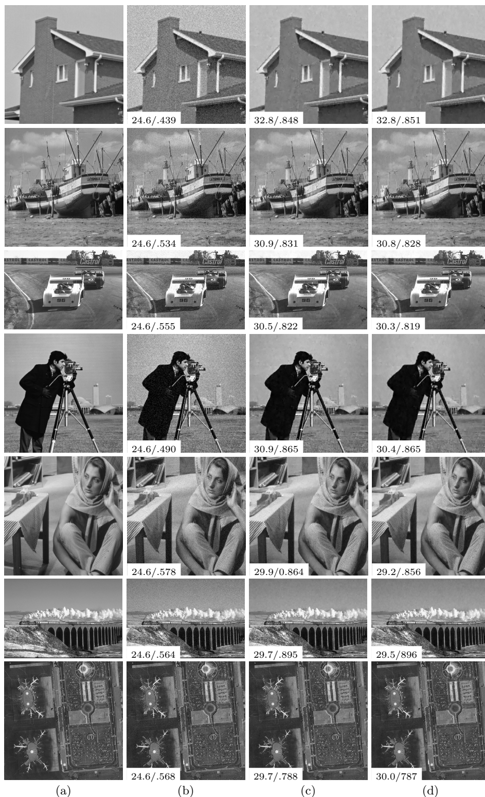
Fig. 2. Denoising results: (a) original, (b) noisy images with \sigma^2 = 15 , (c) results with truncated EM model, (d) results LR-COMP model with PSNR/SSIM. Similar denoising performances are obtained with LR-COMP with a compressed database ten times smaller
