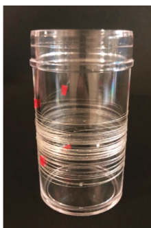
Figure 3. Photograph of the chitosan–TMSA microfiber (ChTMSA001).
