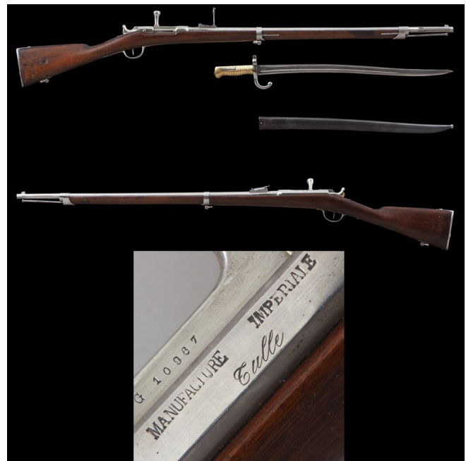
Fig. 7. Photo of the “Chassepot” regulatory breech loading rifle (1866 model) used by the French infantry. Source: https://en.expertissim.com/infantry-rifle-gun-chassepot-model-1866-1770410
