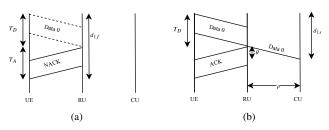
Fig. 4: 1 cycle delay (a) failure and (b) success case (A).
