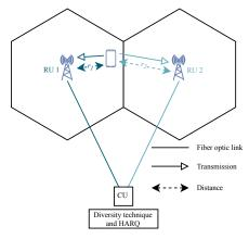
Fig. 3: Architecture B-Multiple receiving BSs (M = 2).
