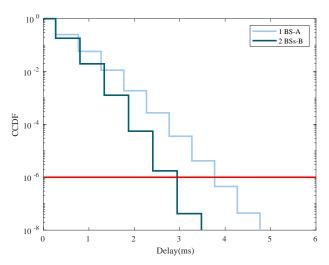
Fig. 10: Delay CCDF for A (with 1 BS) and B (with 2 BSs).
