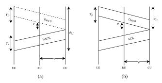
Fig. 5: 1 cycle delay (a) failure and (b) success case (B).
