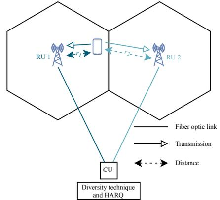
Fig. 3: Architecture B-Multiple receiving BSs ( $M = 2$ ).
