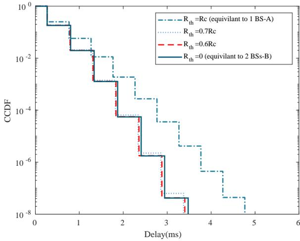
Fig. 12: Delay CCDF with different  $R_{th}$ .
