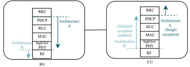
Fig. 8: Flexible split between A and B.
