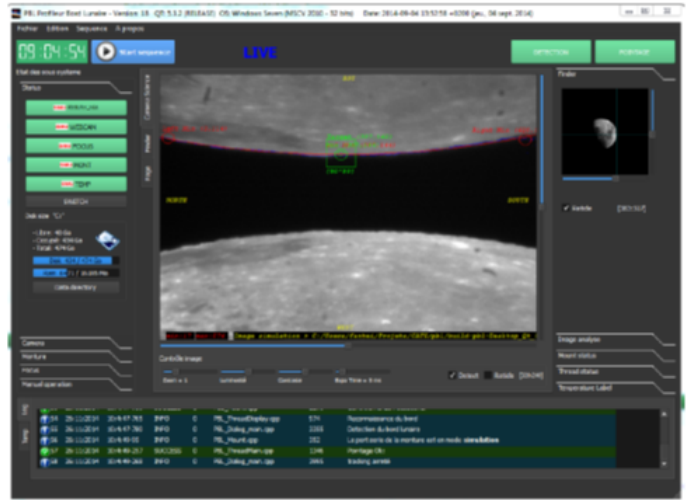
Figure 2. The graphical user interface of the PML instrument showing the two Moon limb images.
