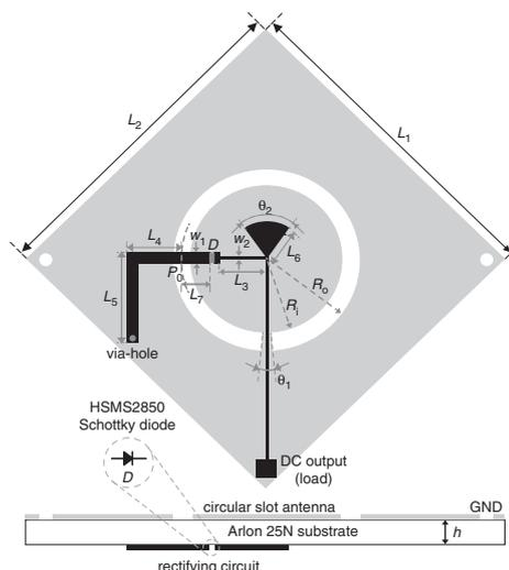
Fig. 1 Geometry of printed shorted annular ring-slot rectenna
