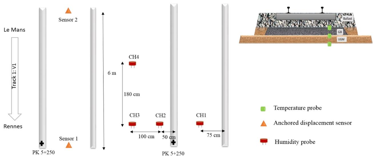
Figure 2 . Instrumentation plan of section 4
