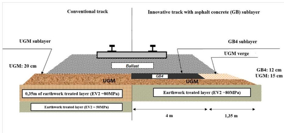
Figure 4. Different structures of the HSL BPL
