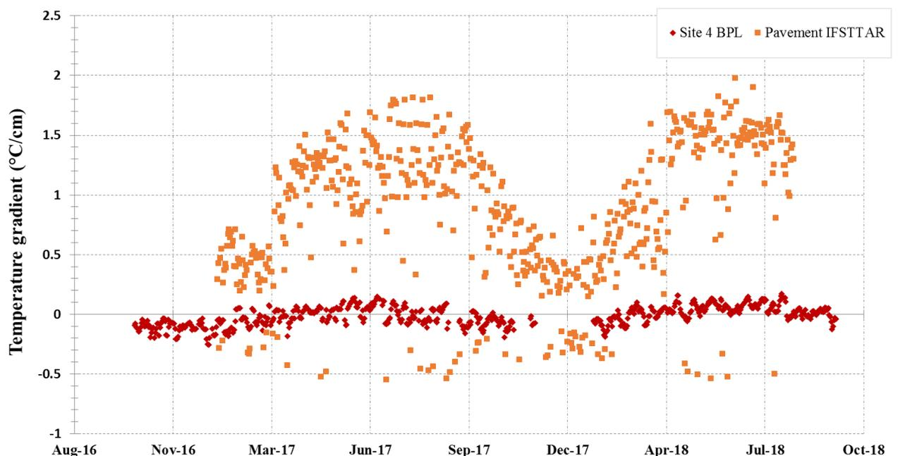
Figure 16. Gradient temperature between top and base of the pavement track's bituminous mixture
