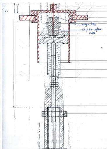
Figure 11. Scheme of the anchored displacement sensor
