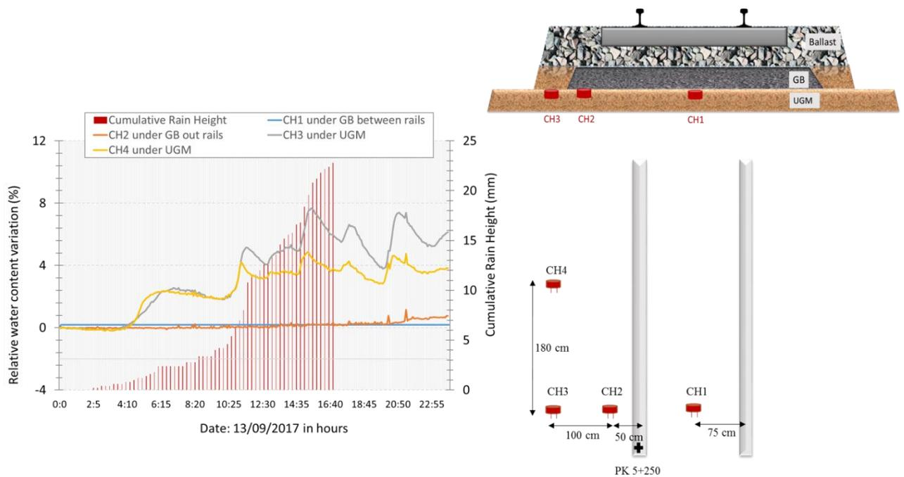
Figure 9. Water infiltration in section 4 (with bituminous sublayer)
