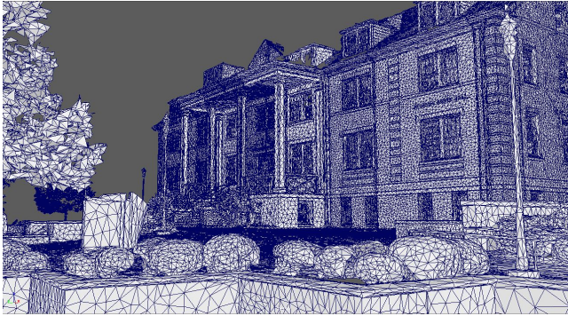
Figure 5: Wireframe shading of a reconstructed building on FAMU campus.
