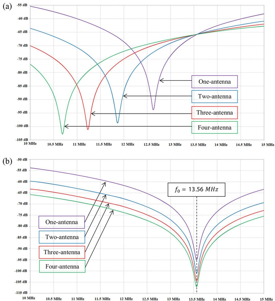
**Figure 3.** Simulated current in the branch of the impedance analyzer in dBA of the textile NFC combiners versus the frequency. (a) Current without taking into account  $C_{SMA}$ . (b) Current with taking into account  $C_{SMA}$  ( $C' = C - N \cdot C_{SMA}$ ).
