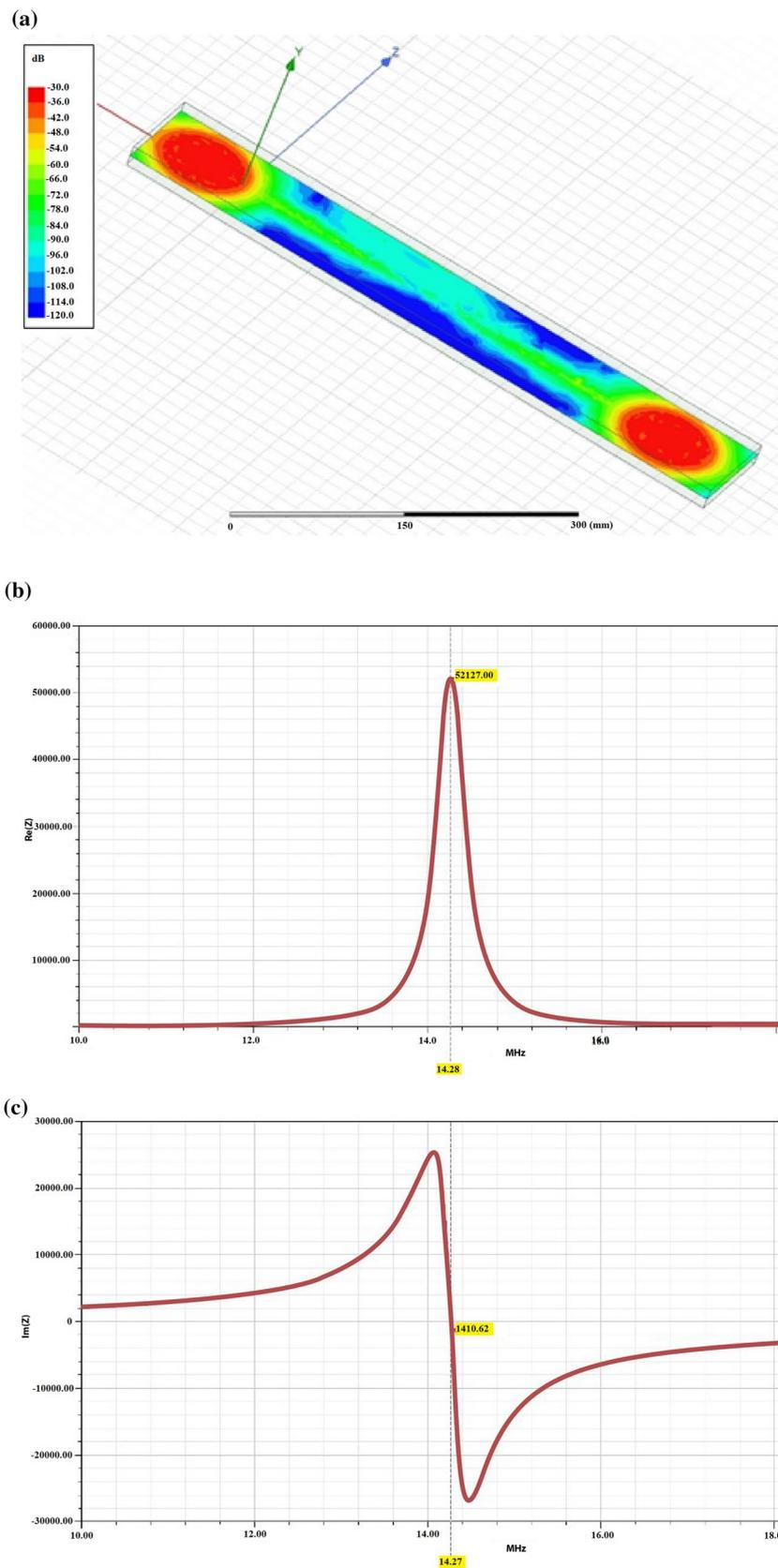
**Figure 6.** 2D cartography of the magnetic field amplitude provided by a 2-coil combiner at 13.56 MHz (a) real (b) and imaginary (c) part of the impedance of a 6-turn coil connected to a 200 mm long two wires rectilinear transmission line.
