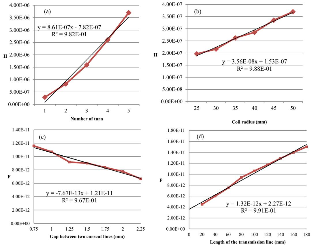
**Figure 7.** Evolution of the coil inductance versus (a) the number of turns and (b) the radius<sup>18</sup>. (c) Evolution of the intrinsic capacity of a textile transmission line ( $l = 100$  mm) versus the gap between its two current lines and (d) the evolution of the intrinsic capacity of a textile transmission line ( $d = 0.75$  mm) versus its length.
