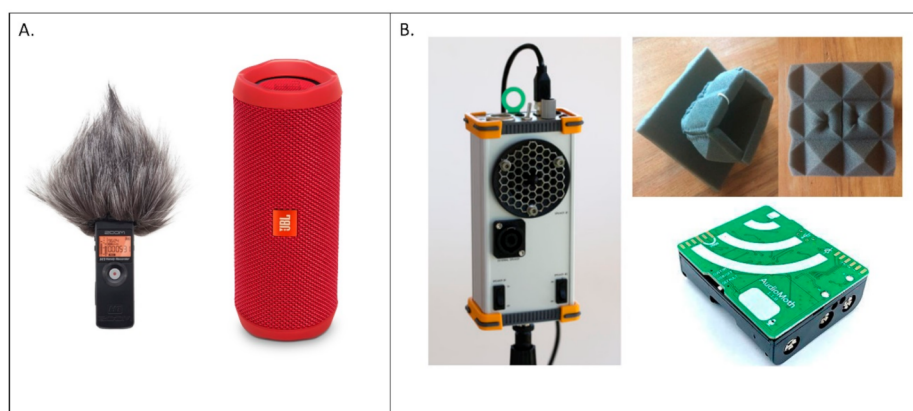
Figure 2. Recorders and speakers used for the trials. (A) ZOOM H1 Handy Recorder equipped with a hairy windscreens (WSU-1). (B) Avisoft UltraSoundGate Player BL Pro 2, AudioMoth recorder and insulation casing with a 26 \text{ kg/m}^3 density pyramid foam (casing = 6 \times 8 \times 7 \text{ cm} ; top = 13 \times 15 \text{ cm} ).
