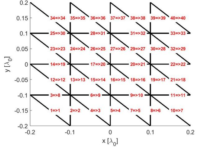
Fig. 1. Sort of the edges. A square plate of area  $L_x \times L_y = (0.4\lambda)^2$  is considered and the sampling steps with respect to the  $x$  and  $y$  directions are  $\Delta x = \Delta y = 0.1\lambda$ . The label  $m \Rightarrow m'$  (or  $n \Rightarrow n'$ ) means that the first number  $m$  indicates the original edge number and the second number  $m'$  gives the new edge number. The integer  $m'$  sorts the edges in ascending order going from left to right and from bottom to top.
