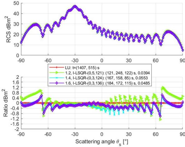
Fig. 4. Top: Bistatic RCS in  $\text{dBm}^2$  versus the scattering angle  $\theta_{\text{scat}}$ . Bottom: Ratio  $\text{RCS}_{\text{I-LSQR}}/\text{RCS}_{\text{LU}}$  in dB scale.  $Q = 0$ ,  $r_{\text{Strong}} = \{1.2, 1.4, 1.6\}\lambda$ ,  $\theta_{\text{inc}} = \pi/6$ ,  $\phi_{\text{inc}} = 0$  and  $\phi_{\text{scat}} = 0$ . The illuminated object is a paraboloid surface, as shown in Figure 3.
