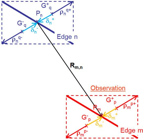
Fig. 13. For a planar surface, interaction of an edge pair  $(m, n)$  and their two facets. The facets are assumed to be identical.
