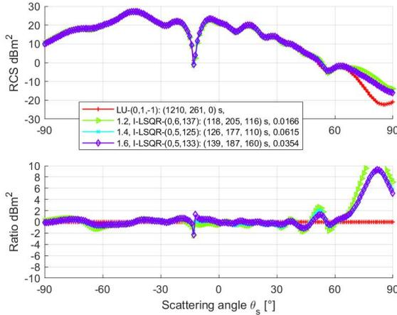
Fig. 7. Top: Bistatic RCS in  $\text{dBm}^2$  versus the scattering angle  $\theta_{\text{sca}}$ . Bottom: Ratio  $\text{RCS}_{\text{I-LSQR}}/\text{RCS}_{\text{LU}}$  in dB scale.  $Q = 0$ ,  $r_{\text{Strong}} = \{1.2, 1.4, 1.6\}\lambda$ ,  $\theta_{\text{inc}} = \pi/6$ ,  $\phi_{\text{inc}} = 0$  and  $\phi_{\text{sca}} = 0$ . The illuminated object is a rough surface, which is plotted in Figure 6.
