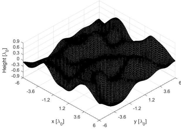
Fig. 6. Surface height versus the coordinates  $x$  and  $y$ .  $L_x \times L_y = 144\lambda^2$ ,  $\sigma_z = 0.3\lambda$  and  $L_{c,x} = L_{c,y} = 1.5\lambda$ . The number of edges is  $N_{\text{Edge}} = 42,960$ .
