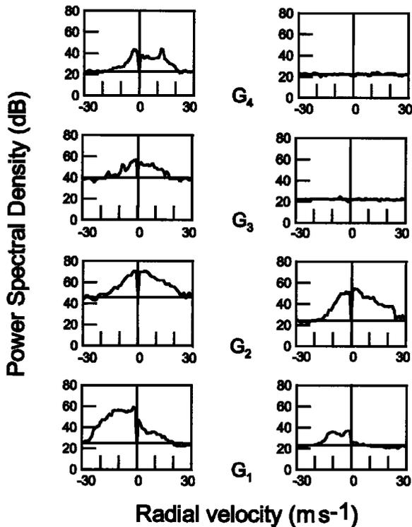
Figure 2. Doppler spectra for gates G<sub>1</sub> to G<sub>4</sub>, integrated for one minute, as a function of radial velocity (positive for targets moving away from the radar). 2a (left): eruption paroxysm (00h03 UT); 2b (right): post-paroxysm (01h36 UT). Horizontal lines correspond to background noise level.
