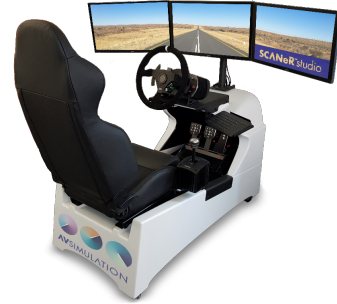
Figure 4: CompactSim, using SCANeR Studio (AVS), adapted to simulate the situation where a human is transported by a CAV.
