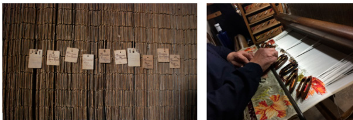
Figure 3. GARIN 1820 atelier: tablet weaving and silk weaver using a brocading shuttle.
