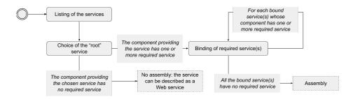
Fig. 2: Building process of a component-based service
