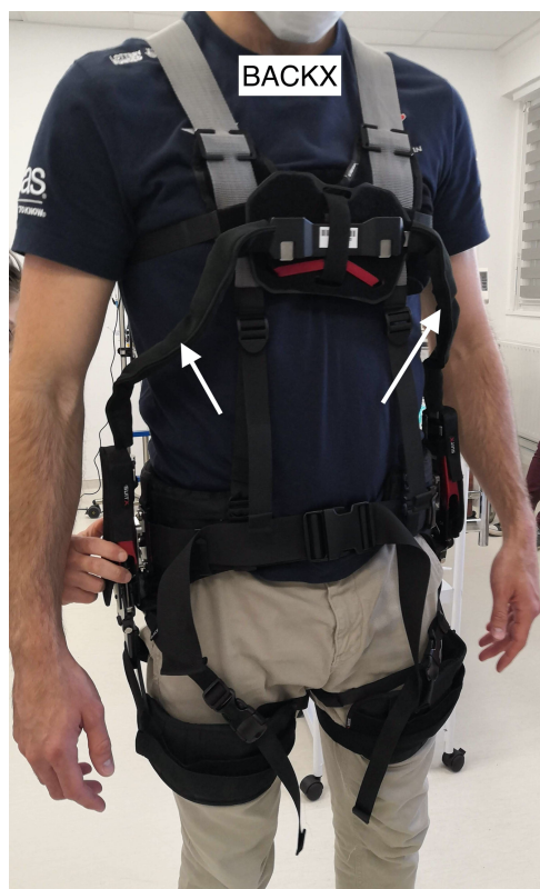
Figure 4 - BackX worn by one participant. The arrows point to the metallic arcs that are constraining the arms during the PP gestures: the participants pointed out that this was one of the main reasons for not choosing to use this exoskeleton for this particular gesture. The BackX was perceived similar to the LAEVO in terms of assistance, but both participants reported that the metallic curved bars from the sternum to the hip were preventing several arm movements necessary to complete the PP maneuver, and as such they felt they could not execute the entire maneuver with this equipment in real conditions.
