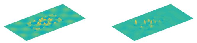
Figure 16: Transverse displacement field (real part) of the plate with  $8 \times 4$  substructures with the floor panel at 125 Hz, obtained with the interpolation strategy. (left) Periodic case; (right) nearly periodic case.
