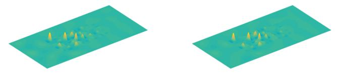
Figure 17: Transverse displacement field (real part) of the nearly periodic plate with  $8 \times 4$  substructures with the floor panel at 125 Hz. (left) Interpolation strategy; (right) FE method.
