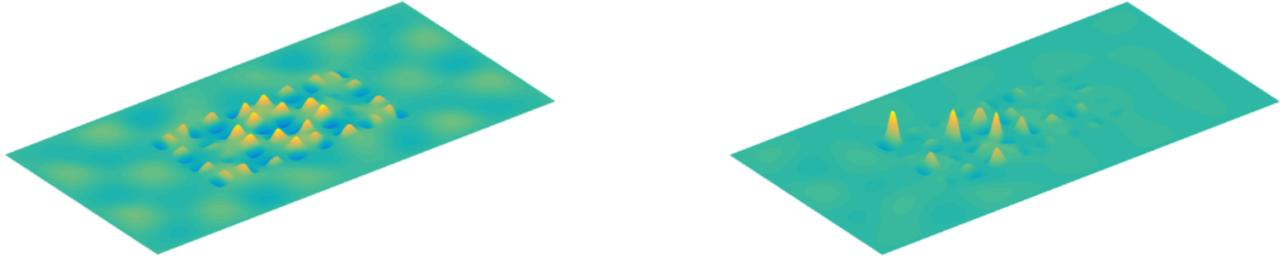
Figure 16: Transverse displacement field (real part) of the plate with  $8 \times 4$  substructures with the floor panel at 125 Hz, obtained with the interpolation strategy. (left) Periodic case; (right) nearly periodic case.
