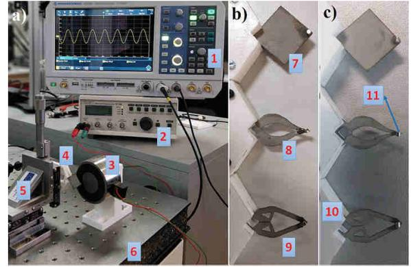
Fig. 6. a) Experimental setup, b) Fabricated designs with magnet direction (1), c) Magnet direction (2). 1: Oscilloscope, 2: Signal generator, 3: Electromagnet, 4: Design, 5: Micro positioner, 6: Anti-vibration table 7: Full plate design 8: Optimized design(1), 9: Optimized design(2), 10: 3D printed supports, 11: Glued magnets
