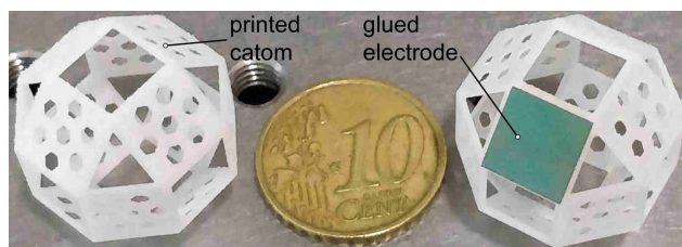
Figure 7. Printed catom's structure and catom with glued electrode.
