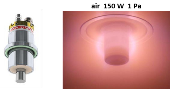
Fig. 1. Aura-wave ECR plasma source (left) and the sustained discharge at 1 Pa in air plasma with 150 W power input (right).
