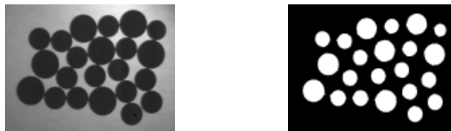
Figure 3. Illustration for separating touching objects in binary image using erosion operator.
