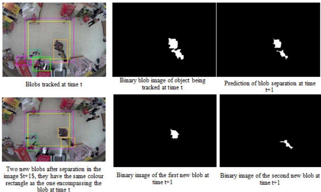
Figure 4. Prediction of the separation of objects at time t+1 using the "erosion" operator.
