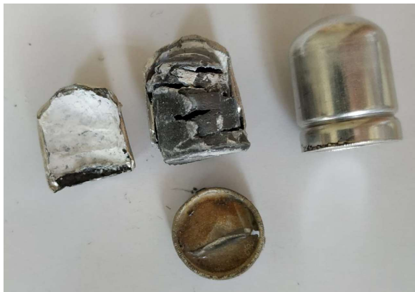
Figure 7 : Capsules opened after ageing test
