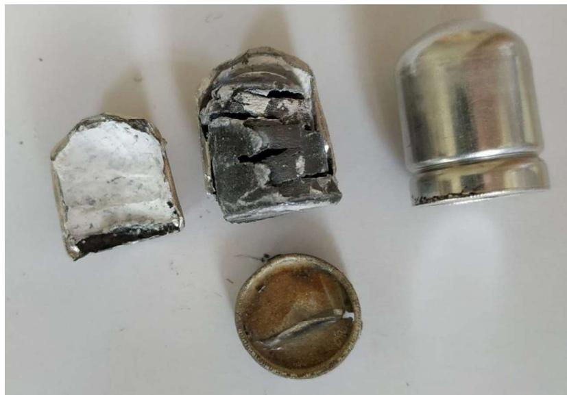
Figure 7 : Capsules opened after ageing test
