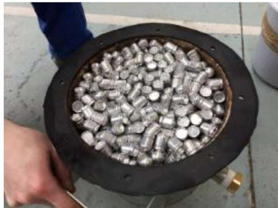
Figure 5 : Storage tank filled with CENG-PCM capsules
