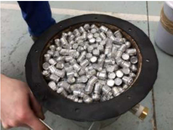
Figure 5 : Storage tank filled with CENG-PCM capsules
