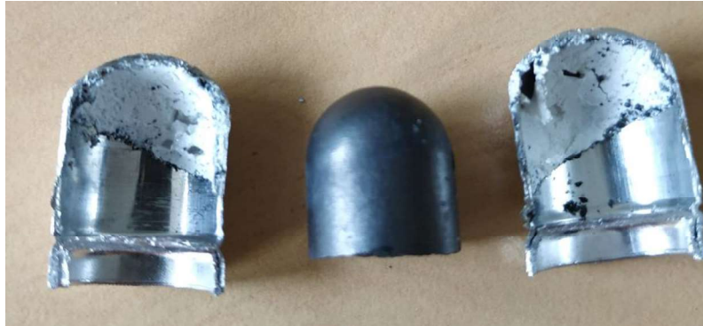
Figure 6 : Picture of an open CENG-PCM-Aluminium capsules
