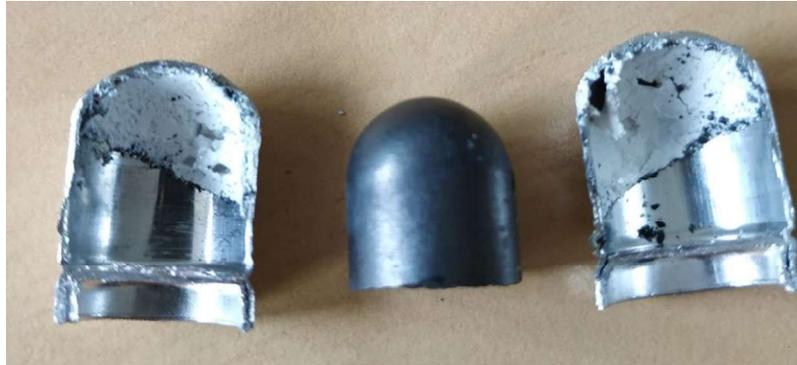
Figure 6 : Picture of an open CENG-PCM-Aluminium capsules
