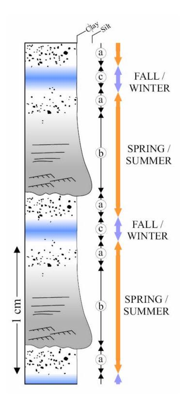
Fig.9: Conceptual model of a typical meltwater-induced fine-grained turbidite sequence. The unitary sequence is composed of two ice-rafted millimetric rich layers (a) spited by a fine-grained turbidite deposit (b). (c) corresponds to millimetric hemipelagic clay intervals.
