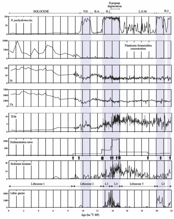
Fig. 5: Time scale of core MD032690 (Guilcher levee): abundance of the foraminifer *N. pachyderma* sin. (%), planktonic foraminifera concentrations (number/g), Ca and Sr records obtained by XRF (cps), Ti/Sr ratio obtained by XRF, sedimentation rates (cm/kyr), frequency of sediment laminae (number/10cm), abundance of coarse (>  $150 \,\mu m$ ) lithic grains (grain/g). Black arrows indicate AMS <sup>14</sup>C dating (Table 2). Highlighted intervals mark polar sea-surface conditions.
