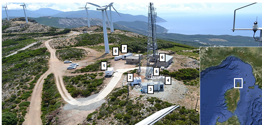
Figure 1. Field site top view, Corsica, France (42.97° N, 9.38° E; altitude 533 m). Measurements performed: (1) VOCs through PTR-MS and online and offline chromatography; (2) OH reactivity; (3) NO x , O 3 , aerosol composition and black carbon; (4) weather, and particle microphysics; (5) HCHO, trace gases and radicals; (6) CO, CO 2 , CH 4 ; (7) trace gases and particle filters; and (8) particle physics. The photo was taken during the installation of the instruments.
