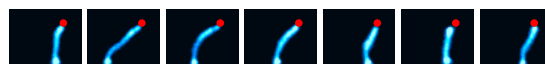
Figure 2: Direct imaging of the plasma discharge using the high-speed camera at 500 fps (false colors). Exposure time is 50 \mu\text{s} to capture a single discharge. The red dots correspond to the tip of the electrode, the bottom of the image to the combustor backplane.
