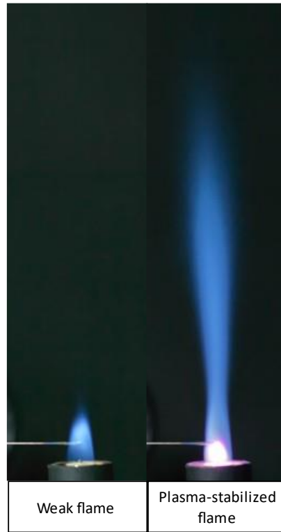
Fig. 4 Photographs without (left) and with NRP discharges applied at 20 kHz (right) in a lean flame
