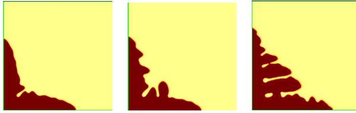
Fig. 10. Final shape of the dendrite with TOL=0.5, 0.75 and 1.
