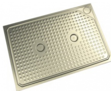
Figure 5: RT44 aluminium panel employed for the both solar chimney prototypes.
