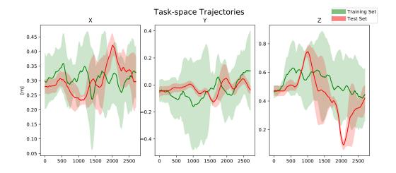
Figure 6: End-effector's trajectories used in the first human-robot interaction scenario: in this case the training set and the test set are belong to different movement primitives.
