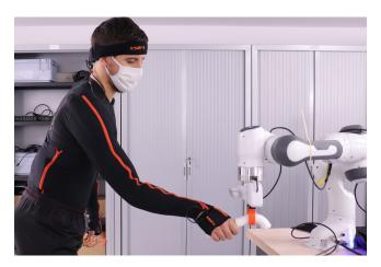
Figure 2: Set-up for the Experiment 1: Human and robot are coupled, robot executes the same trajectory ten times while the human follows its movements.
