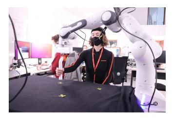
Figure 8: Set-up for the Experiment 3: Human and robot are coupled, robot executes the same trajectory ten times while the human follows its movements.
