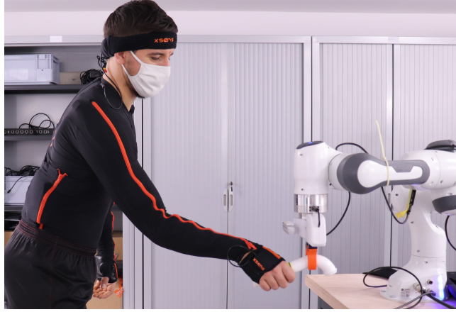
Figure 2: Set-up for the Experiment 1: Human and robot are coupled, robot executes the same trajectory ten times while the human follows its movements.
