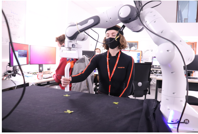
Figure 8: Set-up for the Experiment 3: Human and robot are coupled, robot executes the same trajectory ten times while the human follows its movements.
