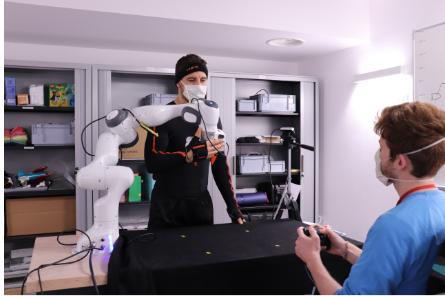
Figure 5: Set-up for the Experiment 2: Robot executes pseudo-random movements while it is controlled by a second operator using a joystick.
