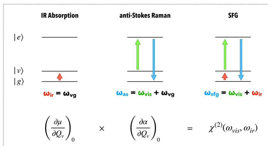
**Figure 10. Vibrational spectroscopies.** Comparison between the three techniques of vibrational spectroscopy: infrared absorption, anti-Stokes Raman scattering and sum-frequency generation. We represent three quantum states  $|g\rangle$ ,  $|v\rangle$  and  $|e\rangle$  for the system, with the same meaning than Figure 7.
