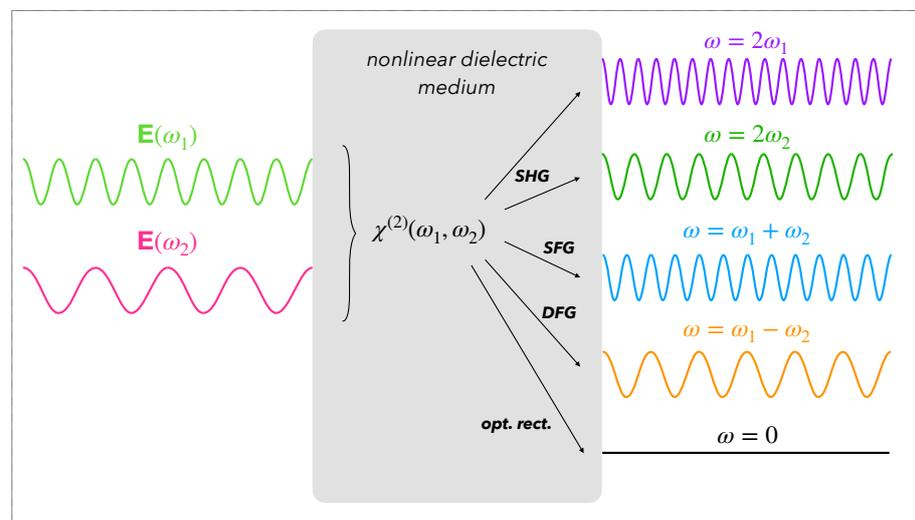
**Figure 4. Second order non-linear optical processes.** Sketch of the processes of second harmonic generation (SHG), sum-frequency generation (SFG) and difference-frequency generation (DFG). These are driven by the second order dielectric susceptibility  $\chi^{(2)}(\omega_1, \omega_2)$  of the material, which couples two input frequencies  $\omega_1$  and  $\omega_2$  to generate new signals.
