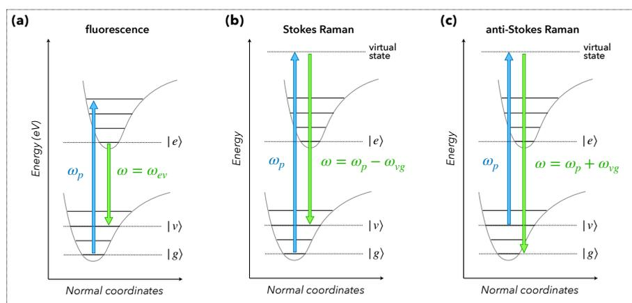
**Figure 7. Fluorescence and Raman scattering.** Illustration of third order non-linear processes: (a) fluorescence, (b) Stokes Raman scattering and (c) anti-Stokes Raman scattering. We note  $|g\rangle$  the ground state,  $|v\rangle$  a vibrational state within the ground state, and  $|e\rangle$  an electronic excited state. The definition of normal coordinates is given in Section 4.1 in the case of molecules.
