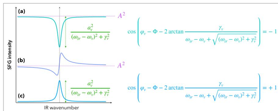
**Figure 12. Interference profiles of SFG spectra.** Typical profiles of the vibrational SFG spectra: (a) in the destructive case, (b) in an intermediate case, (c) in the constructive case. The quantity  $A^2$  corresponds to the non-resonant background. It is not specific to the molecular species but to the inorganic components of the system.
