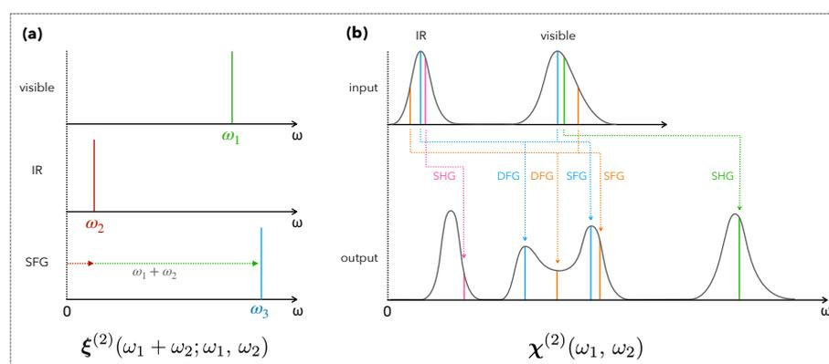
**Figure 1. Mono- and polychromatic picture of second order response functions.** (a) Common description of sum-frequency generation (SFG) from a monochromatic point of view, considered to derive from a 3-argument function. (b) Description of second order processes (SFG, DFG, SHG) from a polychromatic point of view, considered to derive from the 2-argument second order susceptibility  $\chi^{(2)}(\omega_1, \omega_2)$  combining any input frequencies  $\omega_1$  and  $\omega_2$ .
