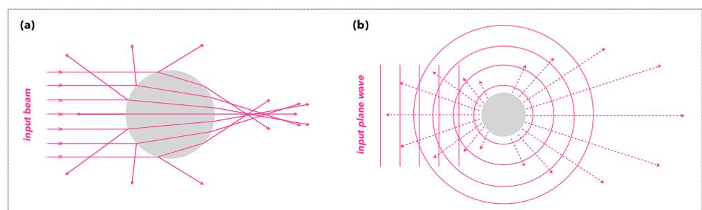
**Figure 3. Geometric and wave description of light scattering.** Sketch of the scattering process, (a) from geometric optics and, (b) from wave optics. The dotted arrows represent the intensity of the scattered light according to the scattering angle.
