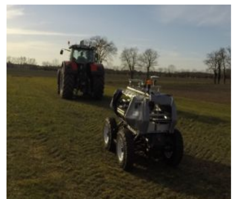
Tractor followed by an autonomous robot (effibot)
