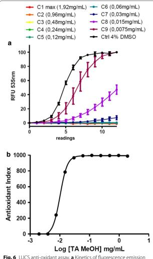
**Fig. 6** LUCS anti-oxidant assay. **a** Kinetics of fluorescence emission recorded under illumination for different concentrations of extract (7.5 10<sup>-3</sup> mg/mL–1.92 mg/mL) using the LUCS assay. **b** Corresponding antioxidant index calculated from RFU values as follows: Al = 1000–1000 (0 f 12 RFUn sample/0 f 12 RFUn control)
