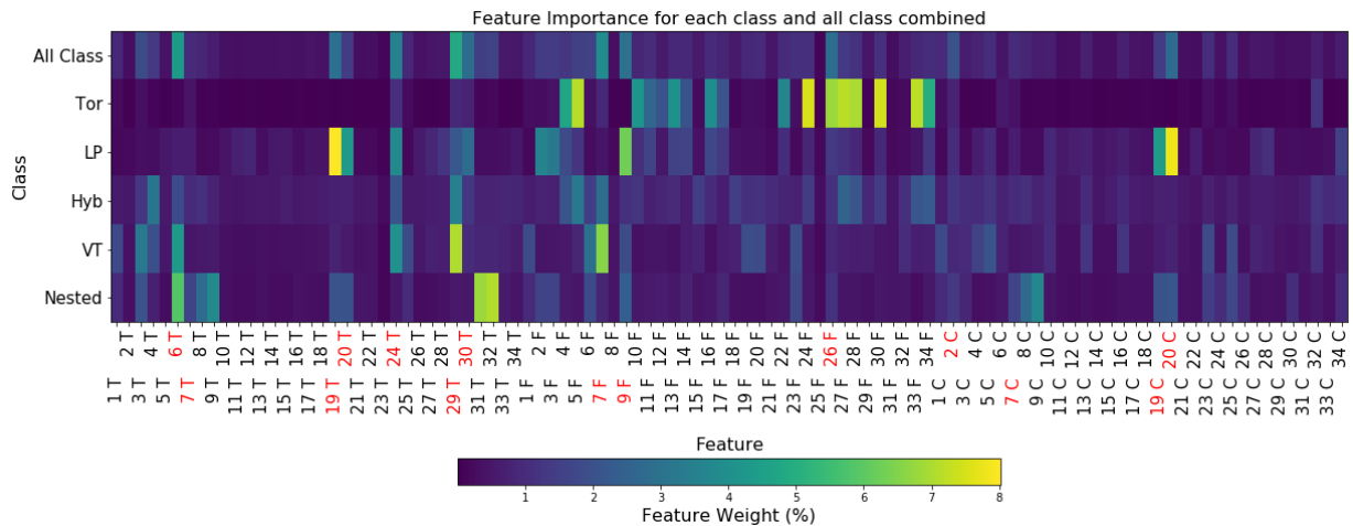
Figure 6: Weights as percentages for all of the features, for each class, and for all classes combined for the volcanic seismicity detected at La Soufrière de Guadeloupe (January 1, 2013, to December 31, 2018; OVSIG-IPGP) determined with the feature importance function in the scikit-learn library. Blue, poor importance in the classification; yellow, important for the classification; red, the 14 most useful features with which the classification is similar to the mean score obtained for the whole feature set.
