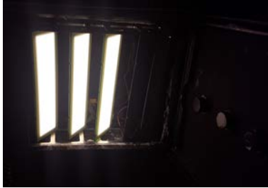
Fig. 6. Inside of a thermal chamber where 3 OLEDs are being tested
