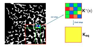
Figure 3: Double local Grid-Block with wall BCs: obtaining the discontinuous tensor in space  $K^*(x)$  and the constant tensor  $K_{eq}$  on the red frame.
