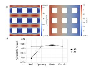
Figure 2: a) Velocity and pressure profile in the case of a periodic geometry A2 with linear pressure BCs ; b) Sensitivity of the permeability (scalar) to the boundary conditions in the case of two periodic geometries A1 and A2.
