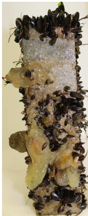
261 262 Fig. 10. Example of sample partially covered with macroorganisms (mussels, ascidians). Samples with 263 macroorganisms attached were not scanned, only biomass was measured.
