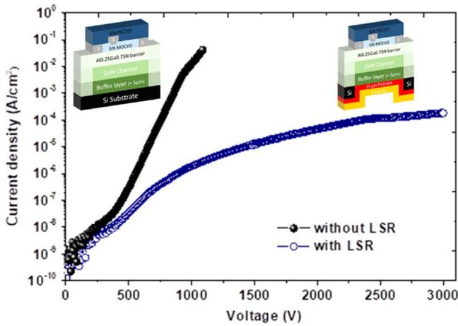
**Fig. 1.** (Color online) Room temperature vertical leakage characteristics of the AlGaN/GaN epitaxial structure with and without LSR.
