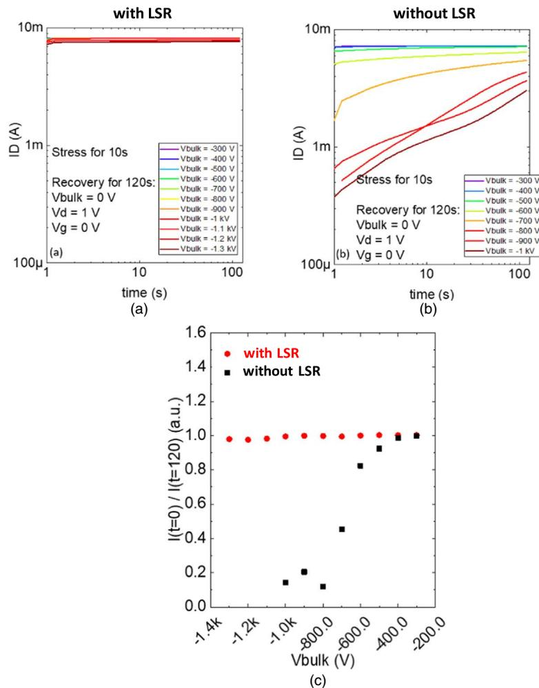
**Fig. 5.** (Color online) Back-gating current transient measurements with various trapping voltages and normalized current after stress as a function of the back bias of AlGaN/GaN MISHEMTs with and without LSR.
