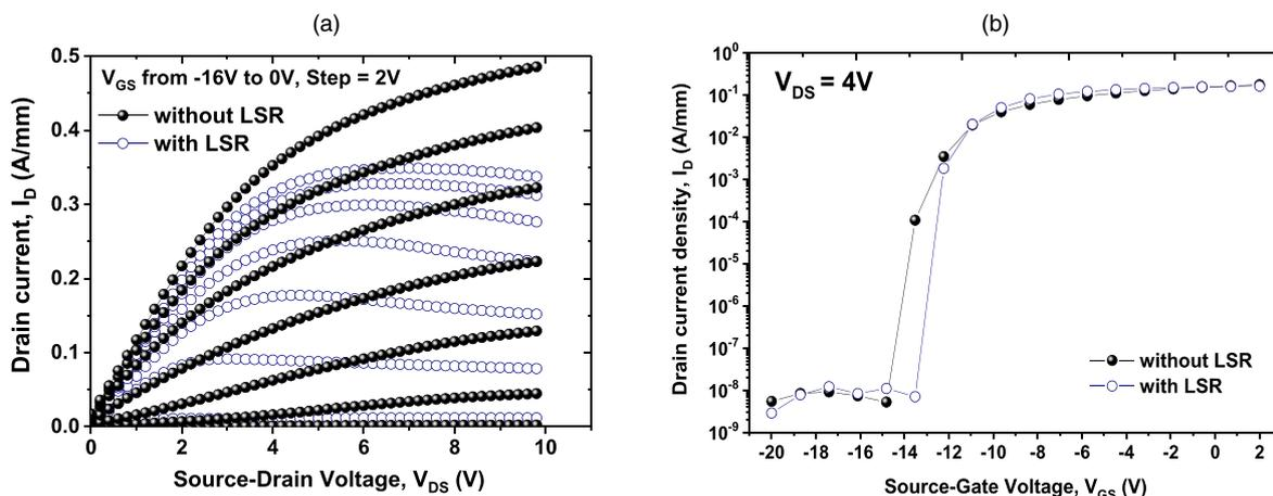
**Fig. 2.** (Color online) (a)  $I_{\text{D}}-V_{\text{DS}}$  and (b) DC transfer characteristics of AlGaN/GaN MISHEMTs ( $L_{\text{GD}} = 5 \mu\text{m}$ ) with and without LSR characteristics.
