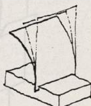
SITUATION INSTABLE DE COMPRESSION -
