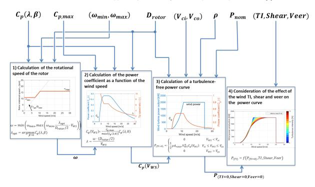
Figure 7: Flow chart representing the main computation steps for the estimation of a power curve from characteristics of a wind turbine
