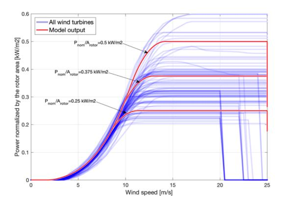
Figure 15: Comparison of all power curves contained in the database (blue curves) with the power output obtained for a power to rotor area ratio of 0.25, 0.375 and 0.5 kW/m2 (red curves)
