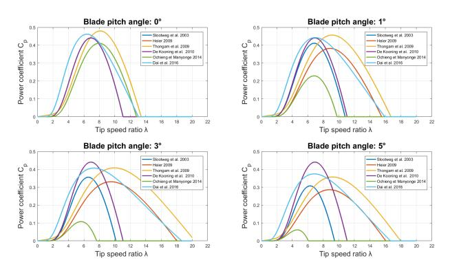
Figure A.16: Comparison of the different  $C_p$  models found in the literature for blade pitch angle values of 0, 1, 3 and  $5^{\circ}$
