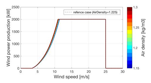
Figure 4: Illustration of the effect of the air density on a power curve
