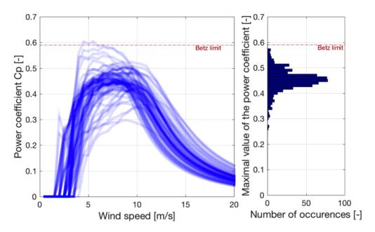
Figure 9: Left: Power coefficient as a function of the wind speed for the power curves available in the windpower.net [44] dataset. Right: distribution of the maximal power coefficient evaluated for all available power curves.
