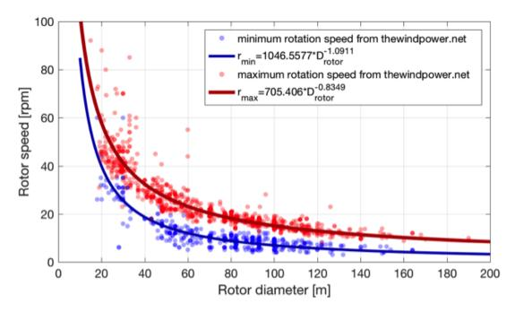
Figure 11: Minimal and maximal rotational speed as a function of the rotor diameter (data source: thewindpower.net [44])
