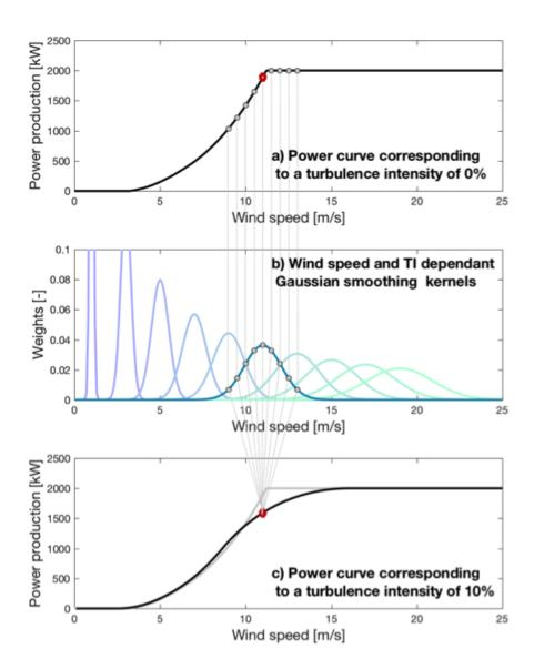
Figure 2: Illustration of the method used to calculate the effect of turbulence intensity on the power curve: the upper, middle and lower plots represent respectively the original power curve, the different Kernels and the final power curve. An example of calculation for a wind speed of 11 m/s is provided.
