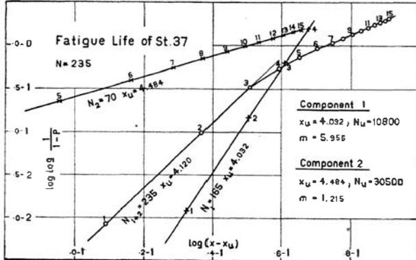
FIG. 6 FATIGUE LIFE OF ST-37 STEEL
