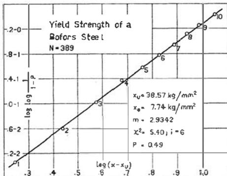
FIG. 1 YIELD STRENGTH OF A BOFORS STEEL
