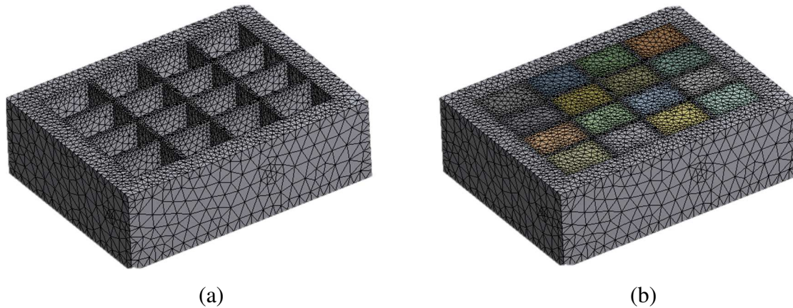
Figure 4. Mesh of the heat sink: (a) without PCM (b) with PCM
