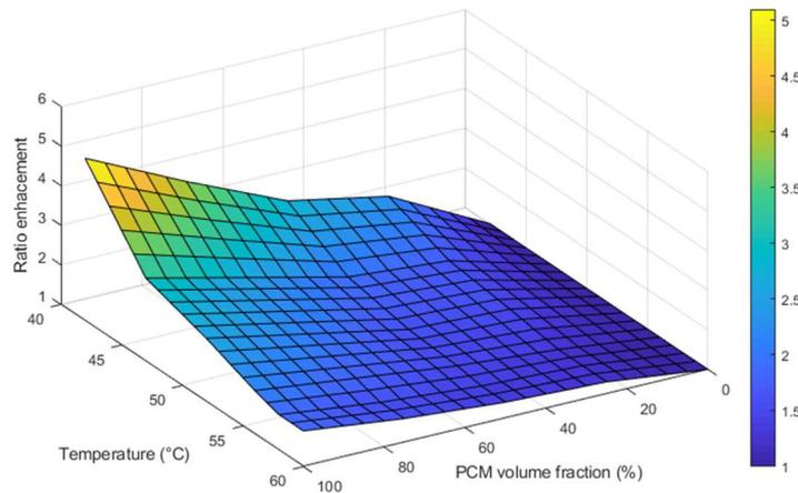
**Figure 13. PCM enhancement ratio of the heat sink matrix for different temperatures**
