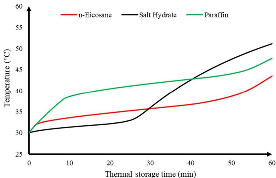
**Figure 9 : Latent process for three PCMs (charging phase)**
