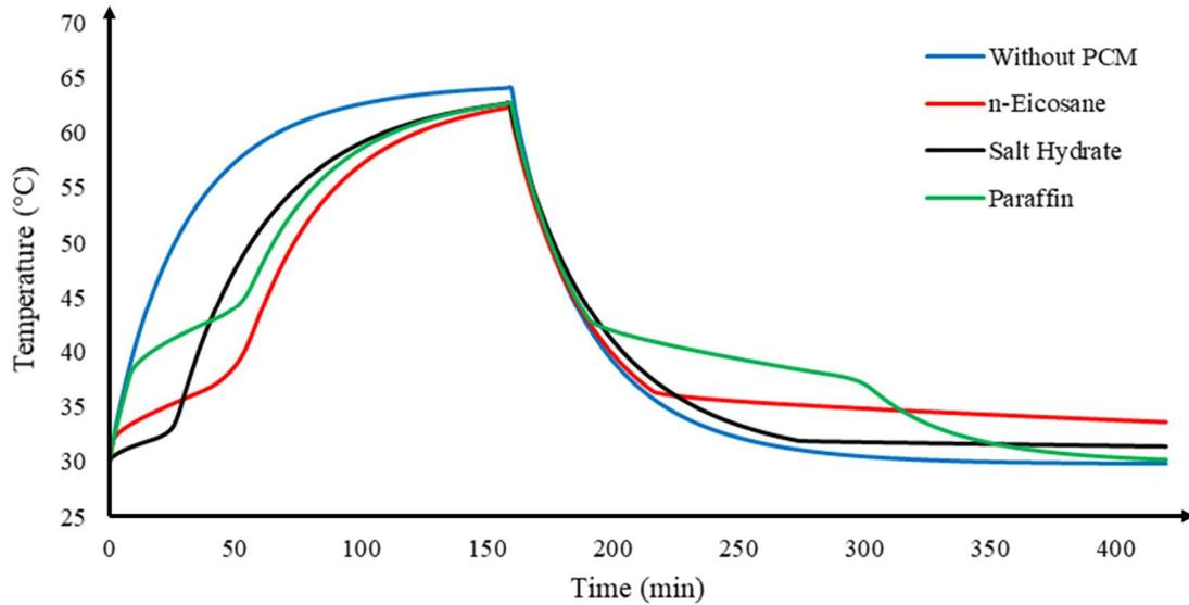
**Figure 8. Melting and cooling temperature profile for three PCMs**
