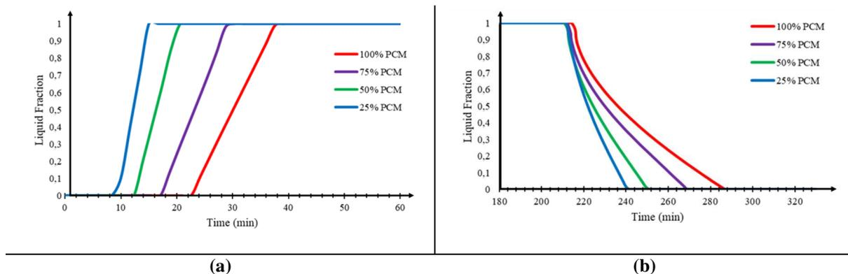
Figure 12. Liquid fraction versus time for different PCM volume rate
