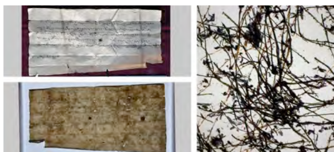
Figs. 16 a, b, c. Document UT/03 from Upper Tshognam written on paper made of Daphne/Edgeworthia sp. fibres with small addition of Stellera sp. fibres. a. Recto side of the document; b. Paper transparency observed against light; c. Fibres observed in 50× magnification.
