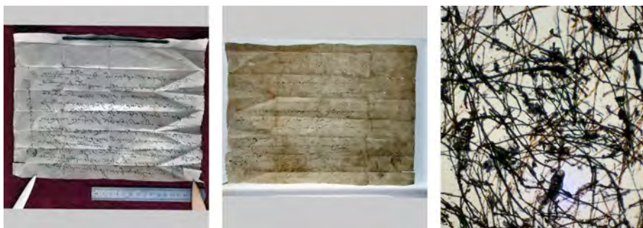
Figs. 42 a, b, c. Document UT/37 from Upper Tshognam written on paper made of Daphne/Edgeworthia sp. fibres. a. Recto side of the document; b. Paper transparency observed against light; c. Fibres observed in 50× magnification.
