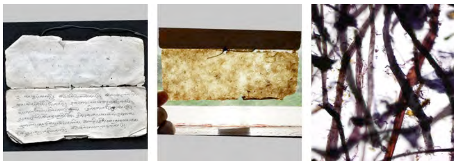
Figs. 12 a, b, c. Document LT/09 from Lower Tshognam written on paper made of Daphne/Edgeworthia sp. fibres mixed with recycled singular fibres of Stellera , cotton and hemp. a. Document in a booklet form; b. Paper transparency observed against light; c. Fibres of Daphne/Edgeworthia sp. with addition of Stellera , cotton and hemp observed in 200 \times magnification.
