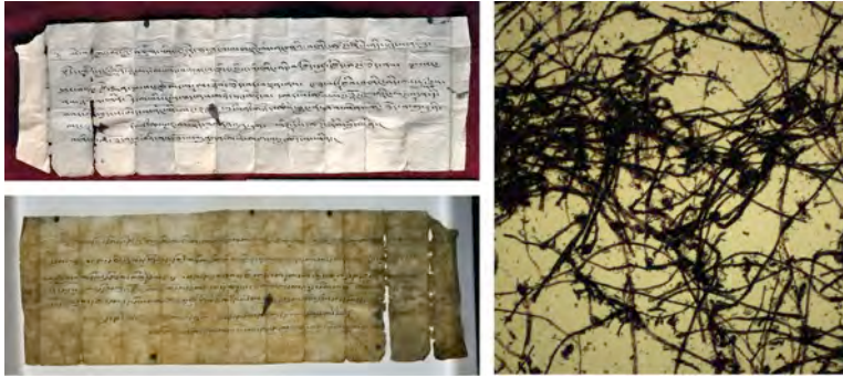
Figs. 17 a, b, c. Document UT/07 from Upper Tshognam written on paper made of Daphne / Edgeworthia sp. fibres with small addition of Stellera sp. fibres. a. Recto side of the document; b. Paper transparency observed against light; c. Fibres observed in 50× magnification.
