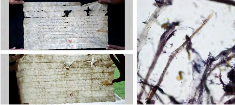
Figs. 9 a, b, c. Document LT/10 from Lower Tshognam written on paper made of Daphne/Edgeworthia sp. fibres mixed with Stellera sp. a. Recto side of the document; b. Paper transparency observed against light; c. Fibres of Daphne/Edgeworthia sp. mixed with Stellera observed in 200× magnification.
