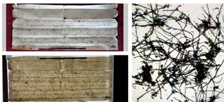
Figs. 26 a, b, c. Document UT/21 from Upper Tshognam written on paper made of pure Daphne / Edgeworthia sp. fibres. a. Recto side of the document; b. Paper transparency observed against light; c. Fibres of Daphne / Edgeworthia sp. observed in 50× magnification.
