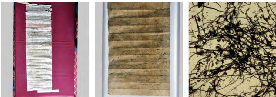
Figs. 41 a, b, c. Document UT/14 from Upper Tshognam written on paper made of mixed Daphne/Edgeworthia sp. and Stellera sp. fibres. a. Recto side of the document; b. Paper transparency observed against light; c. Fibres observed in 50× magnification.
