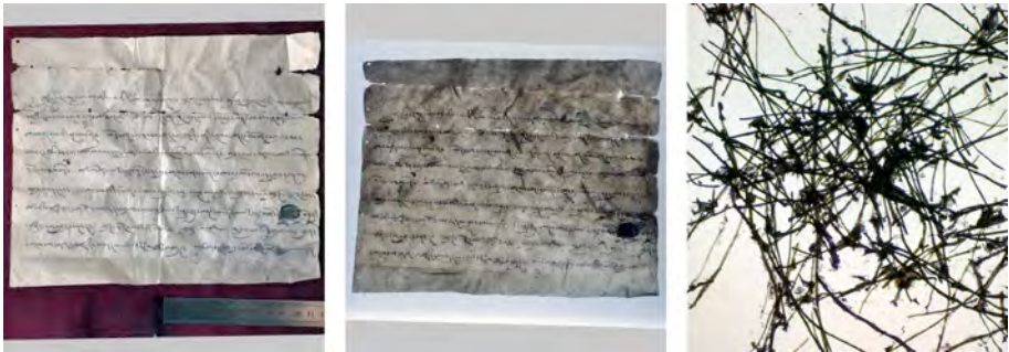
Figs. 10 a, b, c. Document UT/44 from Upper Tshognam written on paper of Daphne/Edgeworthia sp. a. Recto side of the document; b. Paper transparency observed against light; c. Fibres of Daphne/Edgeworthia sp. observed in 50× magnification.
