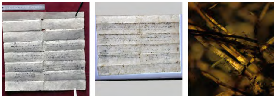
Figs. 14 a, b, c. Document UT/36 from Upper Tshognam written on paper made of Stelleria sp. fibres with small addition of Daphne/Edgeworthia sp. fibres. a. Recto side of the document; b. Paper transparency observed against light; c. Fibres observed in 50× magnification.
