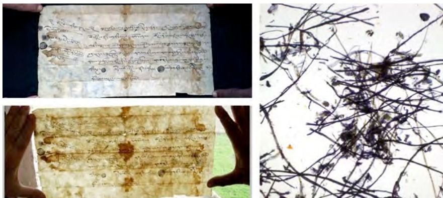
Figs. 20 a, b, c. Document LT/18 from Lower Tshognam written on paper made of Daphne/Edgeworthia sp. fibres with small addition of Stellera sp. fibres. a. Recto side of the document; b. Paper transparency observed against light; c. Fibres observed in 50× magnification.
